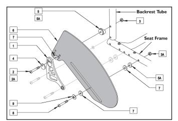
Figure A – Folding Back, Zero Offset
